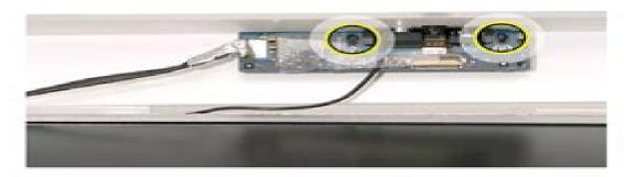
3. Connect the camera and microphone cables.
