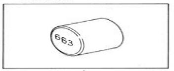
This tool is used for installing the connecting rod small end bearing.
