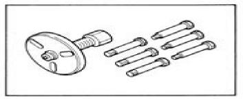
This tool is used for removing the flywheel.
