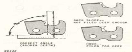
FILING THE CUTTER TOOTH TO THE CORRECT DEPTH is also made easy since the slope of the guide matches the slope of the cutter tooth. This controls filling to the proper depth and prevents a back slope (from not filling deep enough) and a hook (from filling too deep).
