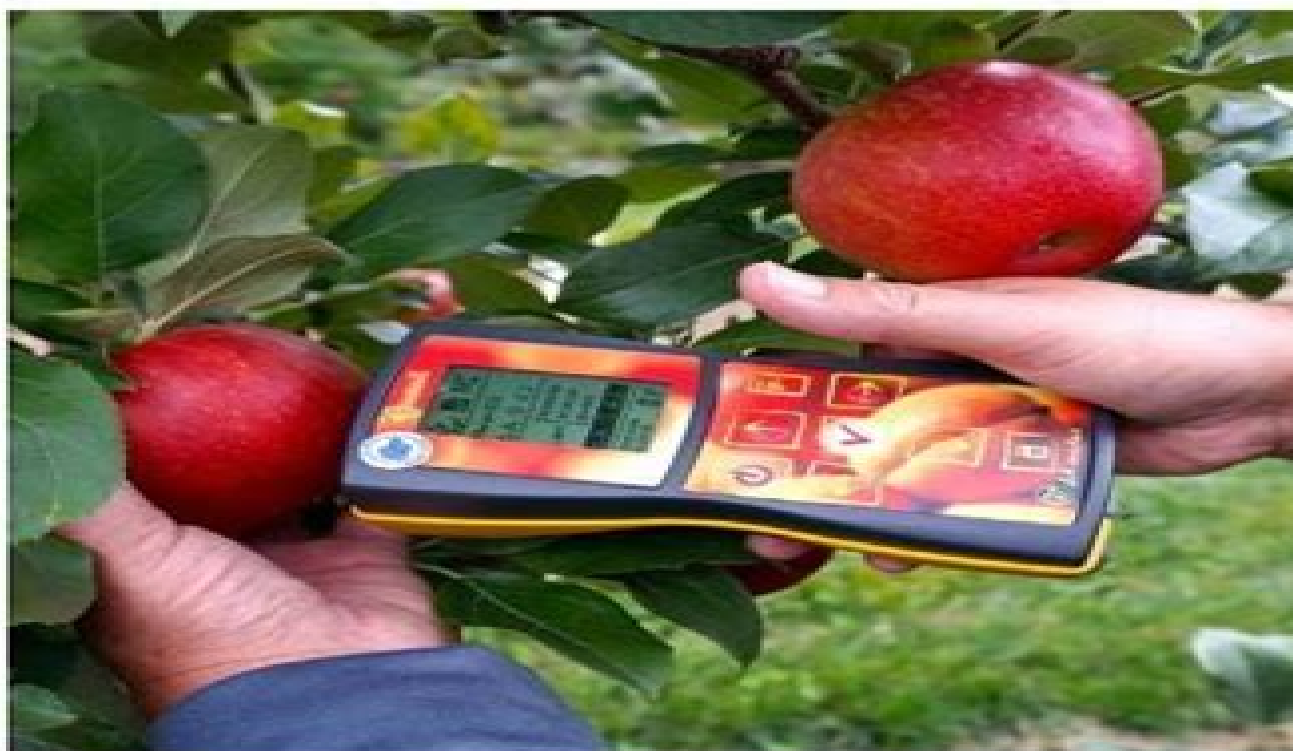
The DA Meter (Turoni, Italy) measuring "Honeycrisp" apple maturity at the UMass Cold Spring Orchard, Belchertown, MA. (Photo: Jon Clements, University of Massachusetts)
