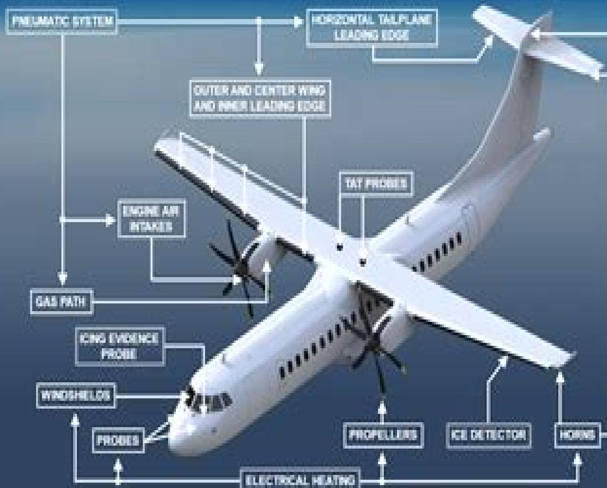
The ATR72-500 ice and rain system permit aircraft operation in icing conditions. Aircraft ice protection is provided by a pneumatic and electrical system for protection of critical areas of the pitotube, engine intakes, propeller blades, windshields, probes and flight control horns. An ice detector is installed under the left wing and alerts the flight crew when ice accretion is sensed by the probe.
