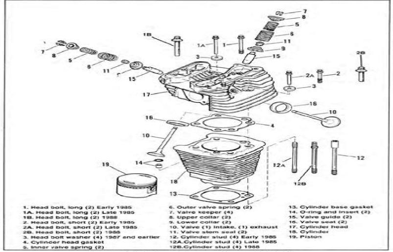
Figure 3-7. Cylinder Head, Cylinder and Piston — Exploded View
