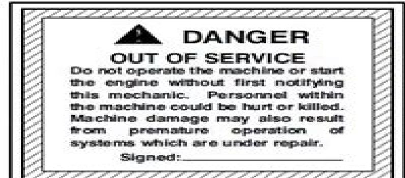
Figure 1-8 Remove the keys from the ignition and post a sign to make others aware of repair activity.
