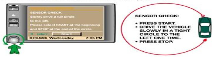
The test requires driving the vehicle in a tight circle at a speed of 6 MPH or less.
