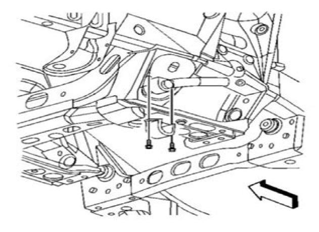
Fig. 3: View Of Stabilizer Shaft, Insulator, Insulator Clamp & Mounting Bolts Courtesy of GENERAL MOTORS CORP.
