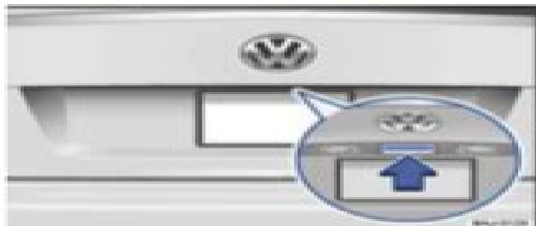
Fig. 28 Opening luggage compartment lid from the outside.
