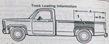
1. Recommended location for cargo center of gravity for cargo weight rating (Pickup Truck).
