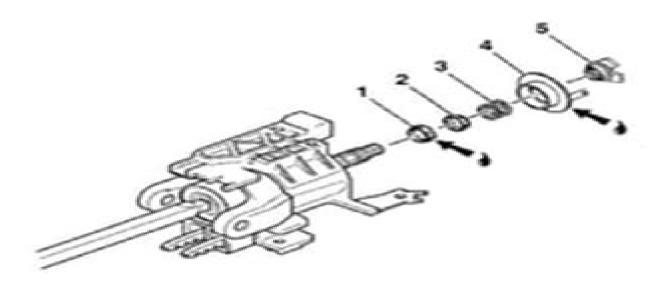
Fig. 24: Installing Following Parts Onto The Steering Column Shaft Assembly (Standard)
