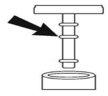
Fig. 4: Identifying FULL COLD Level On Reservoir Cap Courtesy of GENERAL MOTORS CORP.
