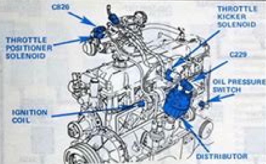
Figure 1 - LH Side of Heavy Duty 4.9L Engine
