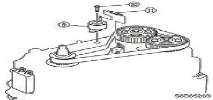
14. Take up the timing belt slack by turning the drive sprocket clockwise at least two full turns.
