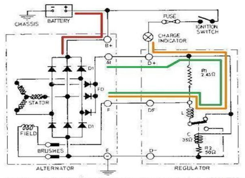
Bosch alternator and regulator circuit diagram. SW-EM
