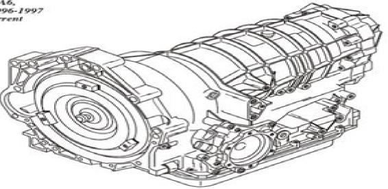
This transmission is manufactured in Germany by ZF and carries the designation ZF-5HP-19...
