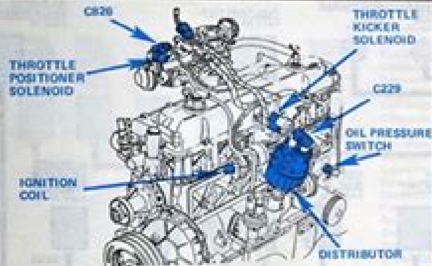
Figure 1 - LH Side of Heavy Duty 4.9L Engine
