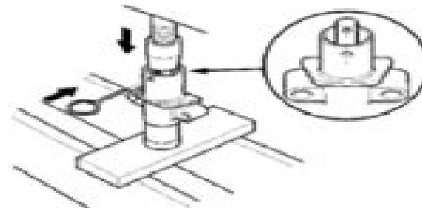
8. Use a hydraulic press to slowly compress the auto-tensioner. Insert a 2.0 mm (0.08 in.) pin through the housing and the rod.
