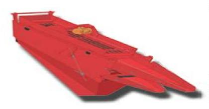
Double Deck: 5'x 10' top scalper deck; 6' x 12' bottom high frequency deck.
