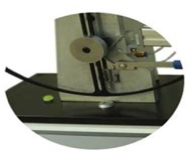
**ASTM D1424 Test Method**
