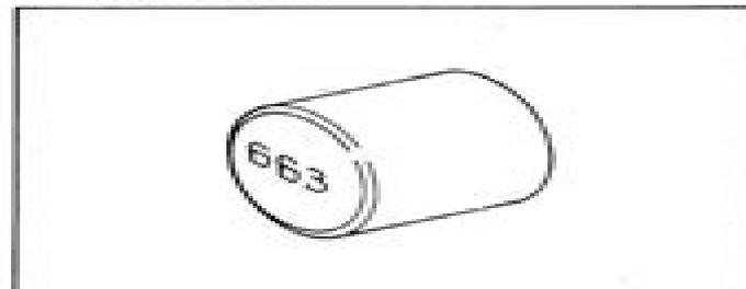
This tool is used for installing the connecting rod small end bearing.
