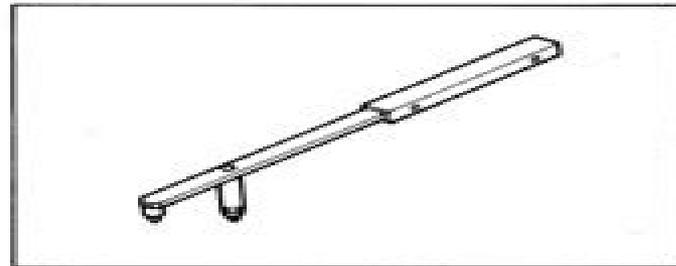
This tool is used for removing and tightening the flywheel securing nut.
