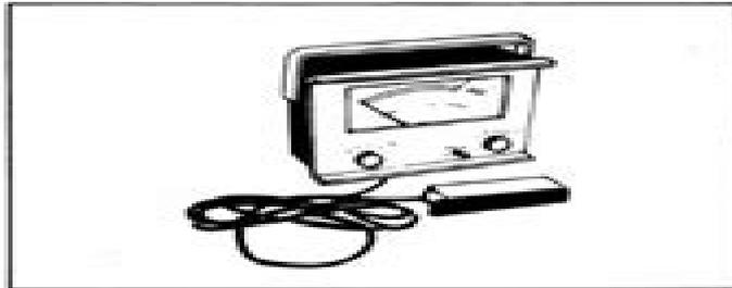
This tachometer is used for checking the engine speed.
