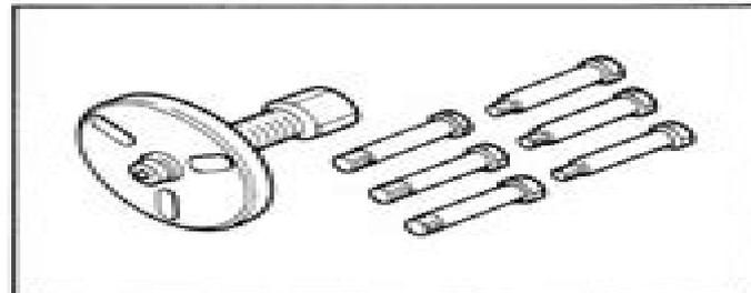
This tool is used for removing the flywheel.
