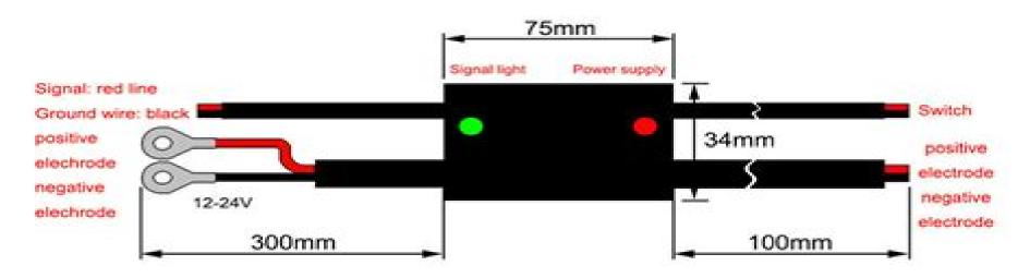
Intelligent detection of vehicle status, engine start, relay standby and flameout off, ensuring that the battery does not lose power
