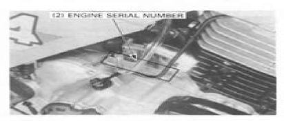
(4) The engine serial number is stamped on the upper side of the right crankcase.
