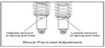
Vehicle loads effect suspension spring pre-load requirements. Use Spanner Wrench (PN 2870872) to adjust pre-load as necessary to avoid bottoming of the shocks.
