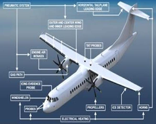
The ATK72-500 ice and rain system permit atcraft operation in icing conditions. Aircraft ice protection is provided by a pneumatic and electrical system for protection of critical areas of the airtrame, engine intakes, propeller blades, windshields, probes and flight control horns. An ice detector is installed under the left wing and alerts the flight crew when ice accretion is sensed by the probe.
