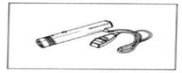
This timing light is used for checking the ignition timing.
