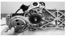
Remove the washer and needle bearing.
