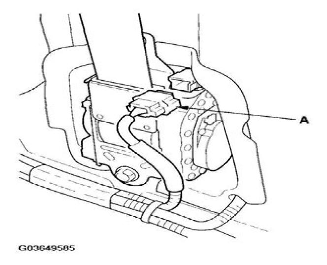
Fig. 31: Disconnecting Floor Wire Harness 4P Connectors From Seat Belt Tensioners (Seat Belt Tensioner) Courtesy of AMERICAN HONDA MOTOR CO., INC.
