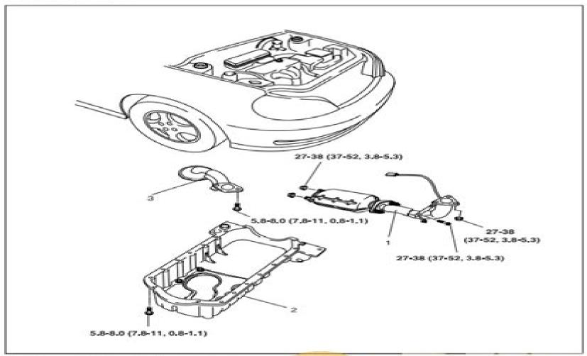
1. Front exhaust pipe & catalytic converter
