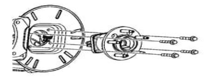
Fig. 1: Identifying Bearing Hub Courtesy of GENERAL MOTORS CORP.
