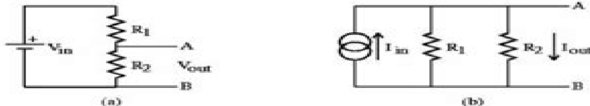
Figure 1.3: Divider circuits: a) voltage divider and b) current divider.
