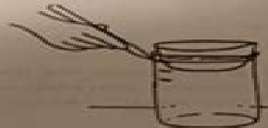
**Step 6:** Retrieve the clay from the bottom, and mold it into a shape that allows it to float. Sketch or describe this shape. Measure the volume of water displaced by the floating clay. Calculate the mass of the water, and record in Table A.
