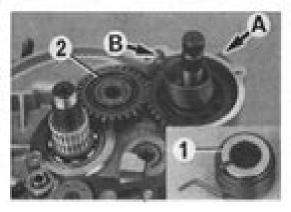
Place internal geared thrust washer and starter gear onto starter shaft. Place driving hub (1) into kick starter spring as illustrated.
